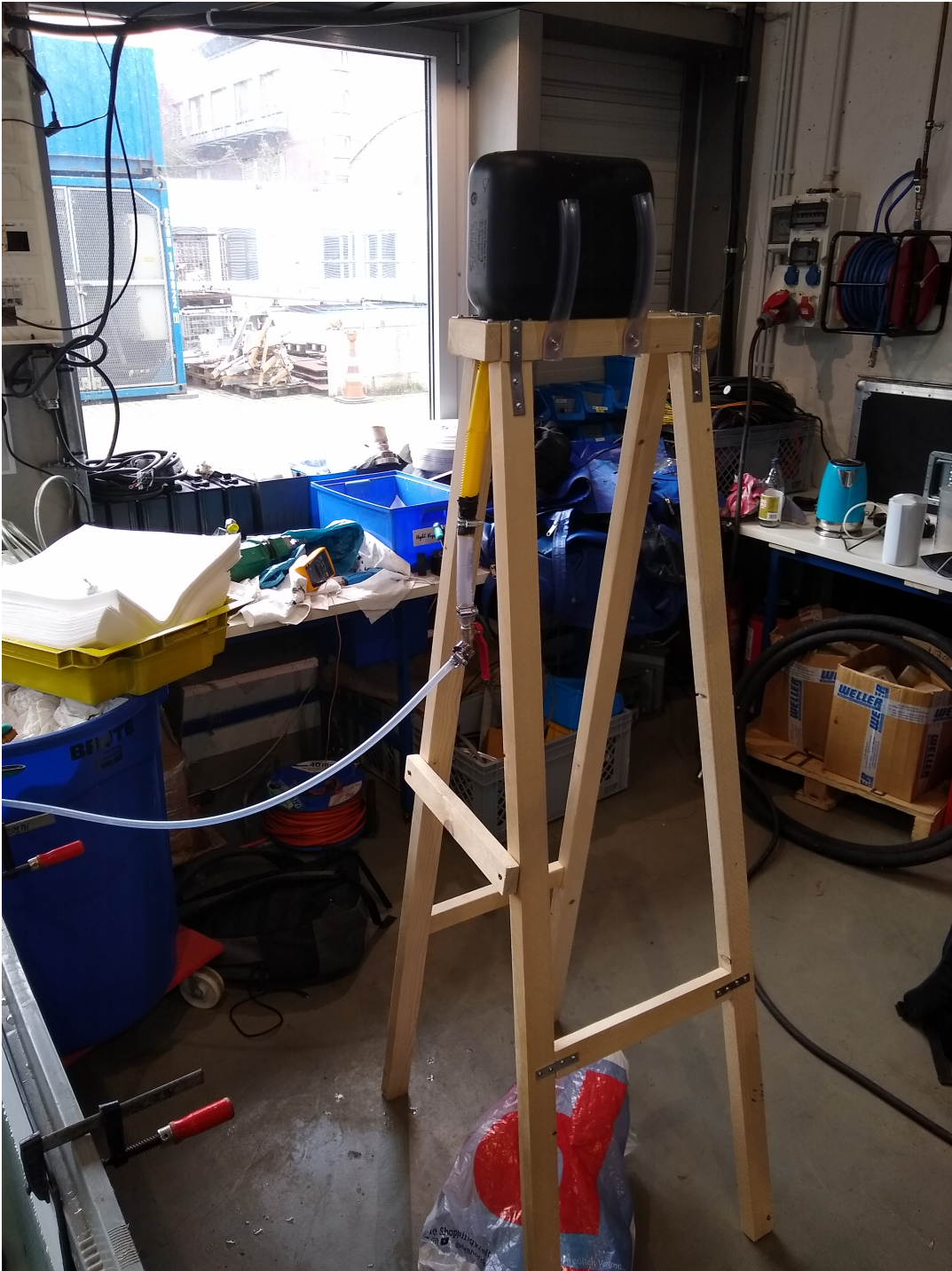
Figure 8: Wood tower and canister of the inflow system for the final test series
