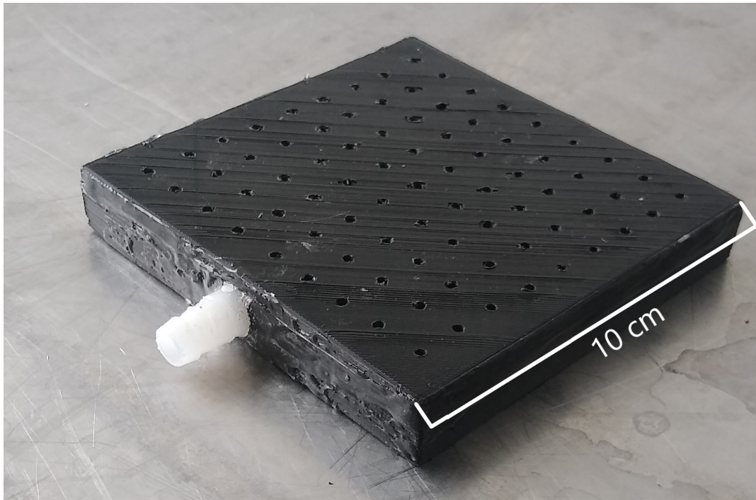
Figure 7: 3D printed inlet used in the final test
