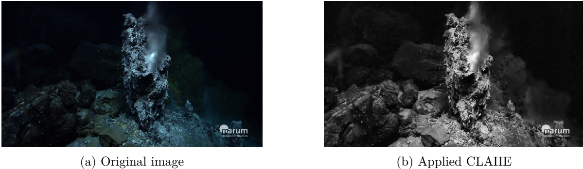
Figure 30: This is an example of how the CLAHE function brightens the dark areas
